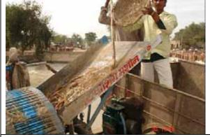
Washer near irrigation canal, the carrots for washing being loaded
