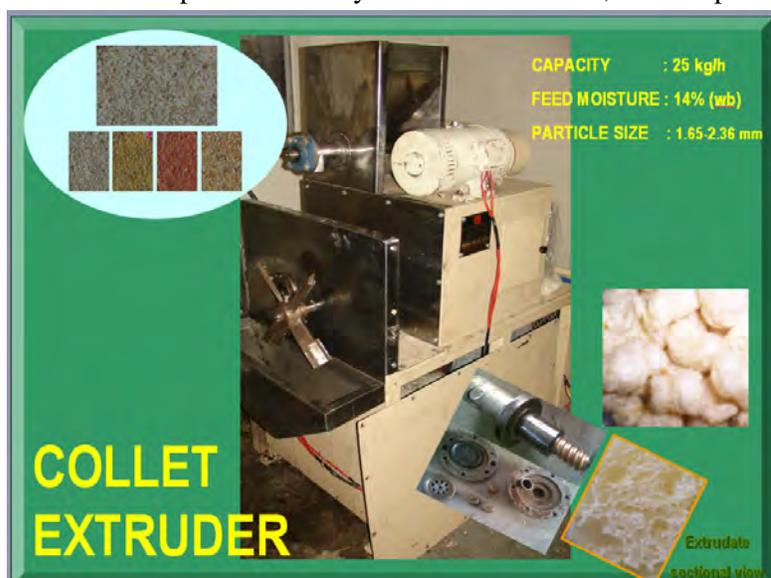
kg/h) and feed moisture (14%, wb), feed particle size (1.65-2.36 mm) were found optimum and kept constant for different protein enriched extruded snack foods. It is attached with a cutter (1 hp DC motor). The feed of required particle size with predetermined formulation can be fed through feeder, which can be regulated by screw auger. The expanded products of 14-20 mm axial diameter can be produced.
