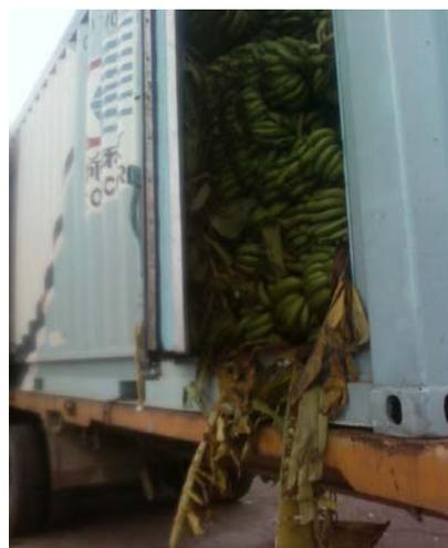
Insulated Ventilated container loaded with banana
