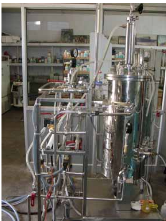
Fermenter of 30 litre capacity with controls for temperature, pH, DO and CO 2 monitoring installed at CIPHET, Ludhiana
