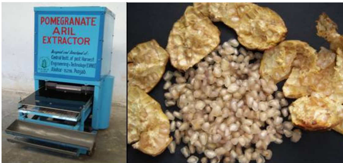
Mechanized version of CIPHET-Pomegranate Aril Extractor and the separated arils from the machine
